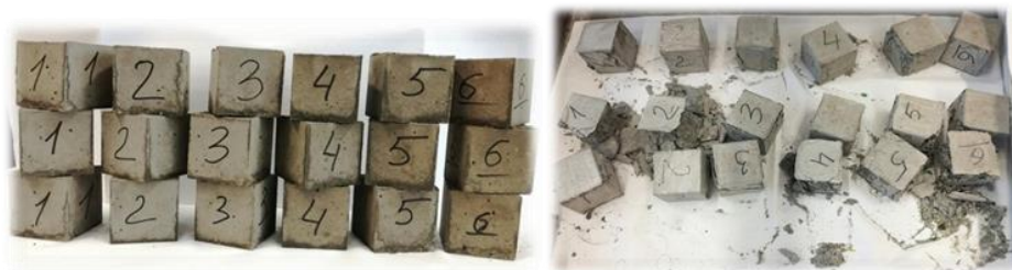
Fig.3. Appearance of concrete specimens before and after testing for compressive strength
